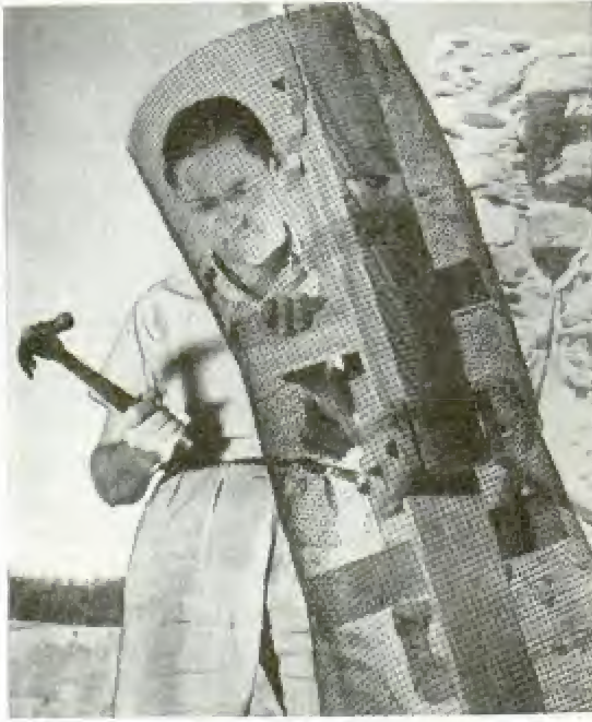
To make a tree trunk, wooden framework is covered with a wire mesh, burlap, plaster of Paris and bark
